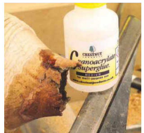
STEP 19. Even though it's the best product for repairing cracks, I don't often use superglue in the workshop as I tend to glue myself together rather than the project! I use the thin version for the small cracks and then the medium one for larger cracks
